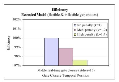
Figure 14: Penalty decreasing efficiency in the extended model (generators being flexible or inflexible)
