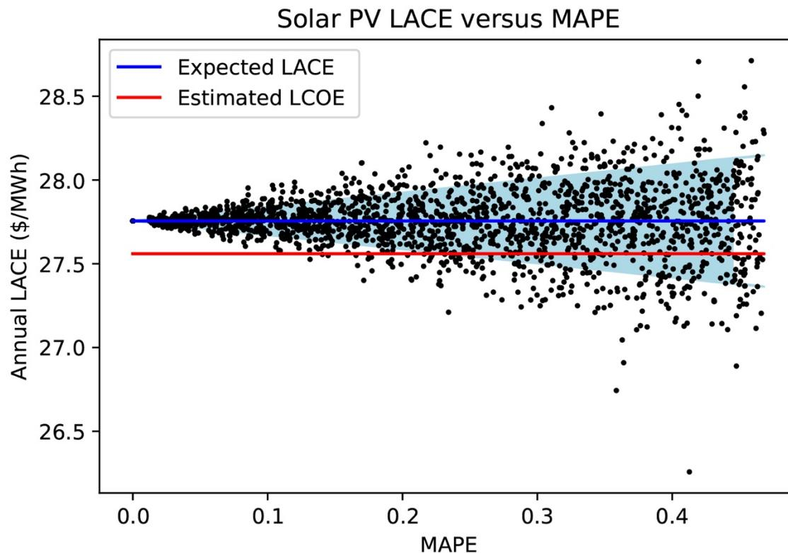
**Figure:** Plot of simulated LACE versus Mean Absolute Percentage Error ( $n = 2000$ ) for an example node in CAISO. The blue line indicates the expected LACE based on 2016 predicted prices, the red line indicates the estimated LCOE, and the light blue area denotes the standard deviation of the simulated LACE computation.
