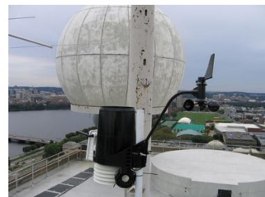
Figure 3.1 Weather station used for data collection. Source: MIT Synoptic Laboratory
